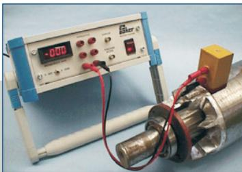
Normally the test system consists of more than one set of sensors to cover a wide range of rotor sizes and slot widths.
